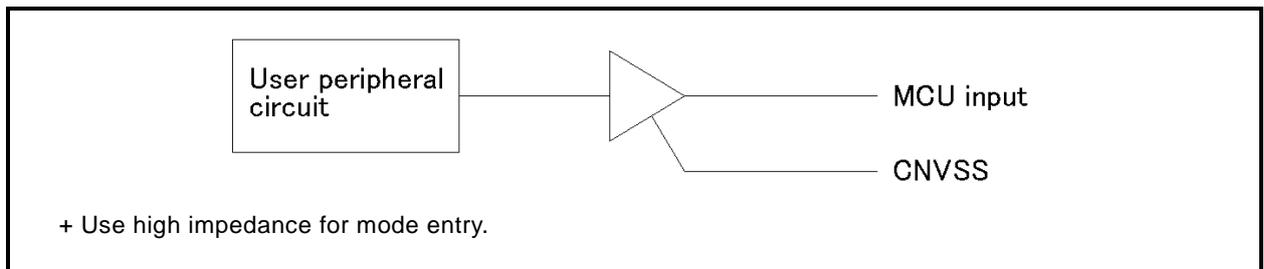
Fig. 4.3: Collision Prevention Circuit Using Three State Buffer
