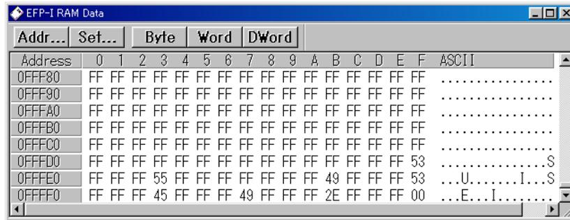
Fig. 6.2: Dump Window (ID Code Setting Data)
